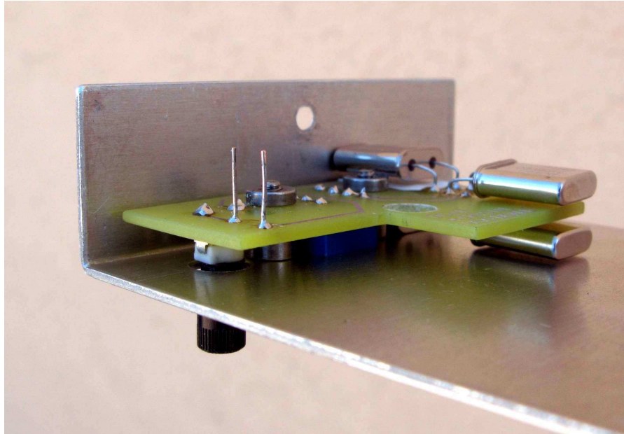
Daughterboard mounted in the top cover with two 4-40 flathead screws and 3/16" thick spacers to bring the dip switch flush with the top cover. Note the two pins to mate to the in-line pin sockets.
