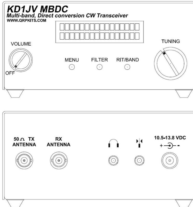
The decals are applied the same as model decals. Cut around each group of text or symbols you wish to apply. It doesn't have to be perfect as the background film is transparent. Apply the decals before you mount anything to the chassis. Use the above picture to get the correct spacing around the holes and cutouts, as it is very easy to do a great decal installation and have a portion covered up with a knob
