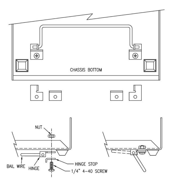
The chassis bail consists of a bail wire, right hinge, left hinge, two hinge stops, two 1/4" 4-40 screws, and two nuts. Prior to mounting the PCB into the chassis, use the above illustration as a guide and attach either of the side hinge assemblies to the chassis, as shown, with nut to the inside. Then slide in the bail wire and secure the other hinge assembly, with the nut to the inside.
