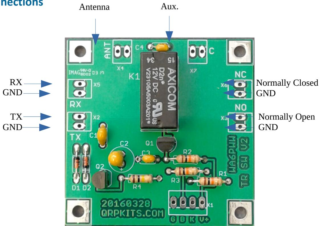
The Antenna, RX and TX as well as the second switched pair (C, NC and NO) are as shown above.
