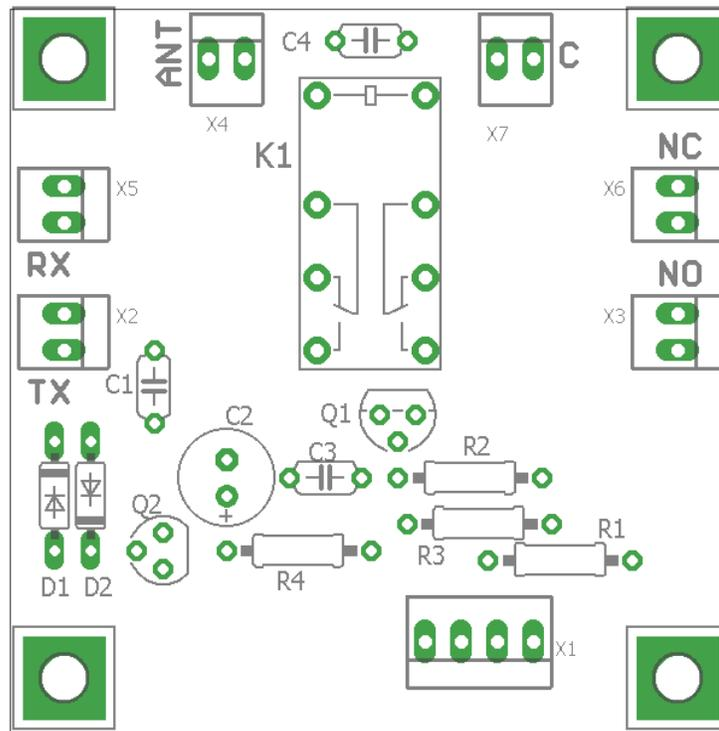
Note: Pin 1 of X1 is the pad closest to the X1 Label (on the right above) and is the connection point for 12V power. The leftmost pin (4) is ground connection.
