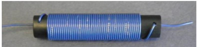
Wind the coils counting one turn each time the wire passes the starting point. Keep the wire as tight as possible during winding.
