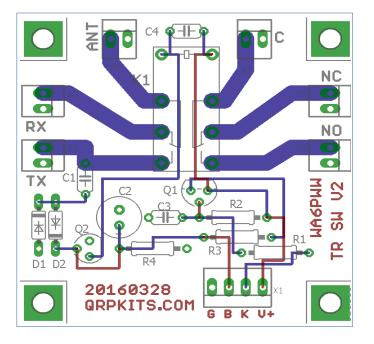
Note: Pin 1 of X1 is the pad closest to the X1 Label (on the right above) and is the connection point for 12V power. The leftmost pin (4) is ground connection.
