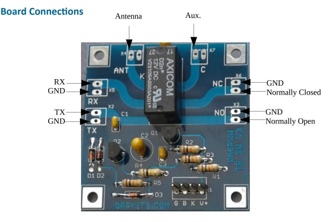
The Antenna, RX and TX as well as the second switched pair (C, NC and NO) are as shown above.
