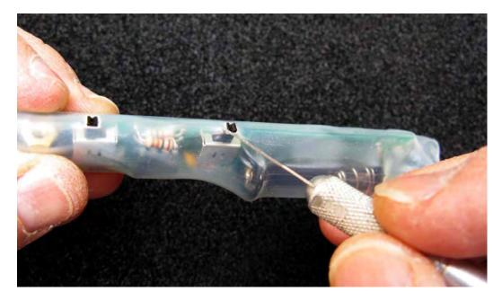
• Use an Xacto knife, and trim around as shown. This picture shows after the trimming. This will provide for a nice finished look when complete.
