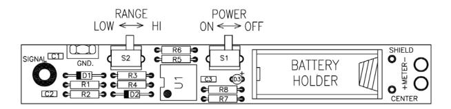
All components are soldered on the silk screened side of the board. Solder all the resistors in place, following the above guide and the silk screened locations. Bend the leads 90° and lay the resistors down flat, there are no vertically mounted resistors. Trim all leads after soldering. If you have any doubt as to the correct value, double check them with your VOM. R5, 6, 7 are 1% resistors, so they have 5 color bands.
