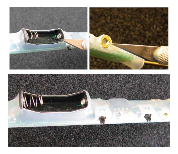
• After the shrink tubing has cooled, use a razor knife to carefully trim around the switches, so they have full travel. Carefully trim the access to the battery compartment, alligator clip connection point, and around the probe end as needed.
