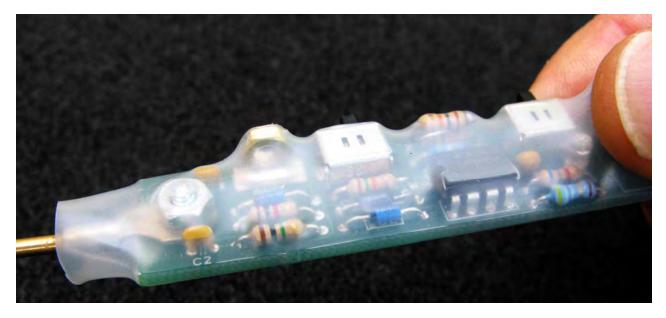
• Finish shrinking the tubing until it pulls down to touch the surface of the components and the bottom of the pcb. Be careful around the battery holder, it is especially sensitive to overheating. You are just looking to insulate and protect the components and pcb! Do not overheat.
