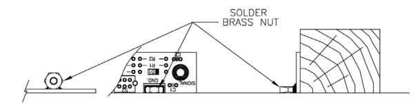
• Solder the nut, flush to the side of the board. Use something square to position the board up against, I used a small piece of wood, and lie the nut down 90 degrees to the board. This will be the alligator lead connection point used later. Do not get any solder inside the threads of the nut.
