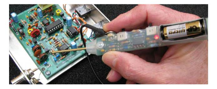
Install the battery, and you are ready for use. The 12v battery was selected for it's small size. It is an inexpensive, readily available battery, used in devices like garage door openers, etc. The assembly only draws a few mA, but still do not leave the power switch on, when not taking measurements.
