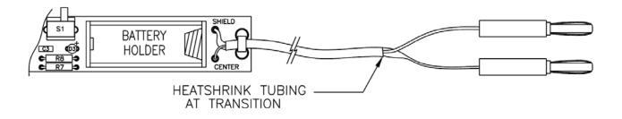
• Solder the center conductor to the pad marked CENTER, and the shield to the pad marked SHIELD. Secure the coax to the pcb using the cable tie supplied
