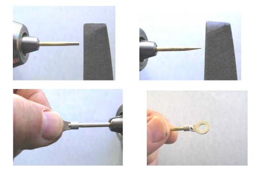
File a contact point on one end of the 2" long, 3/32" brass rod as shown. File down the other end of the brass rod to accept the other #4 ring terminal, and solder it in place. An electric drill makes it easy, but you can do it by hand as well.
