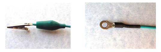
Slide the plastic boot back from the alligator clip and solder the lead to the clip. Sometimes these are crimped only, and can lose conductivity. Replace the boot. Cut the 3/16" dia. x 2" L. heat shrink tubing in half and place one piece over the loose end of the alligator clip lead. Solder the lead assembly to one of the #4 ring terminals, and shrink the tubing to the transition from the ring terminal to the lead. Color may vary from picture. Set it aside for later assembly.
