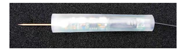
Slide the complete assembly into the shrink wrap, battery end first. Center it into the piece provided. It gets a little tight after going over the top of the potentiometer shaft and past the mode switch. Take your time, it will fit.
