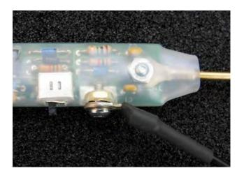
Attach the alligator lead assembly with the remaining 4-40 x 1/4" pan head screw, and lock washer. The proper order is, 4-40 screw, ring terminal, internal tooth lock washer, attached to the brass nut. Do not over tighten or you will break the brass nut off the pcb.
