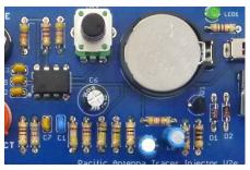
Bend the leads down at each end of the resistor to fit the board holes.
